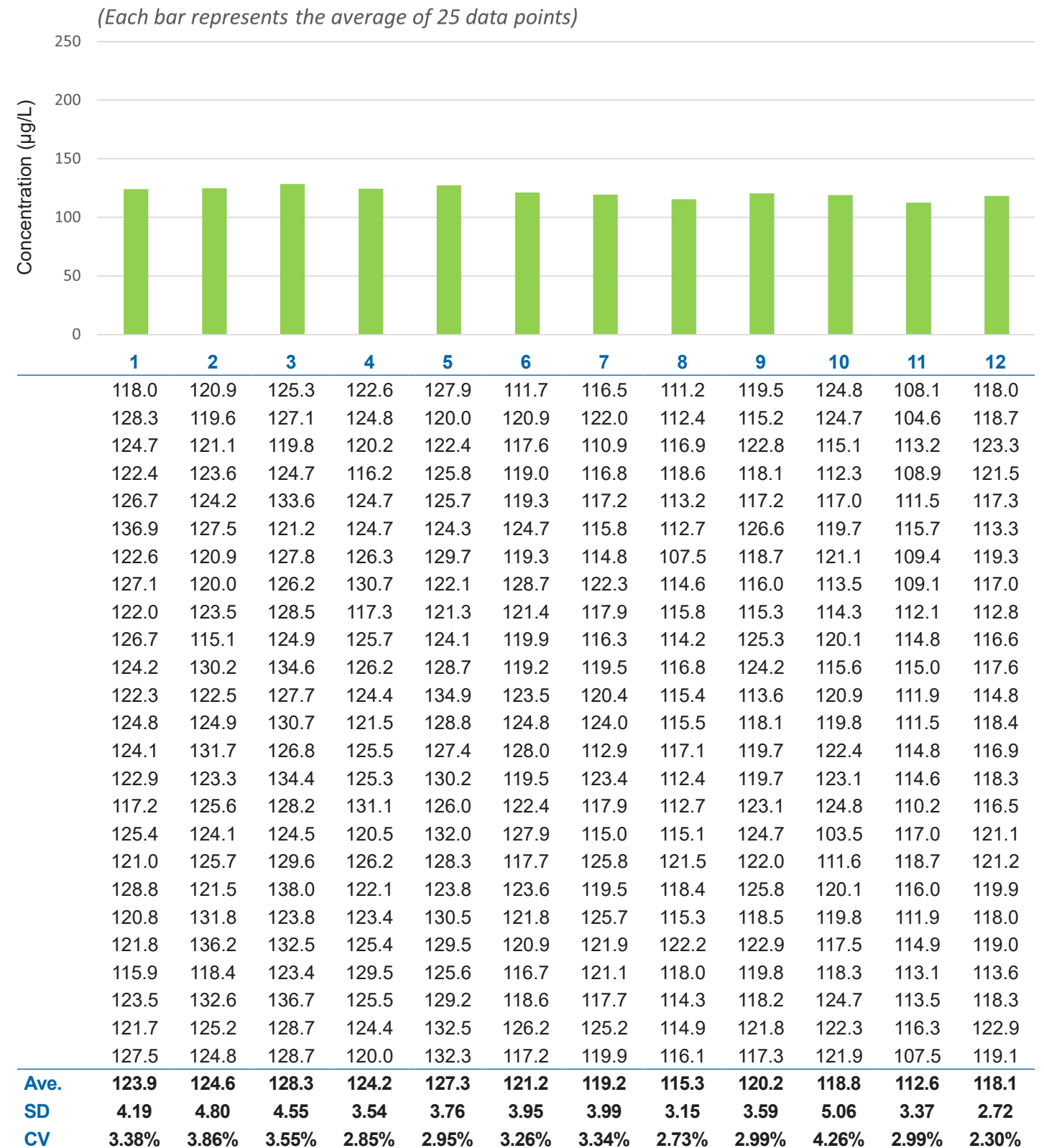
Figure 10. Low concentration for selenium measured by ICPMS (m/z 78). Each number 1-12 corresponds to a batch. The graph above shows the average, and the numbers below show the individual sample data from the batch.
