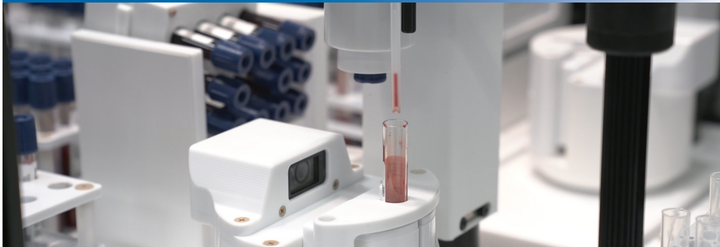
Figure 2. TRAXStation Clinical takes up a whole blood aliquot for automated preparation in a 96-well microplate.
